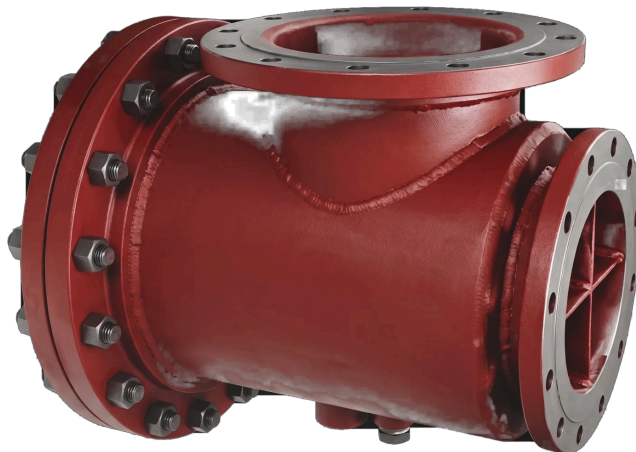
Cast suction diffuser. It replaces the elbow, the strainer and the straight entry pipe on a pump suction with one component.
