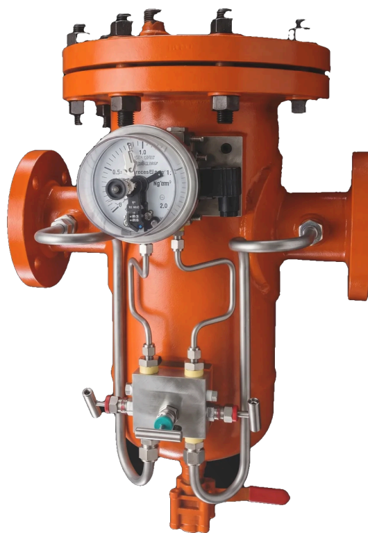
Cast basket strainer with differential pressure gauge, instrument manifold and drain valve fitted. Cast and fabricated construction are both covered by this catalogue.
