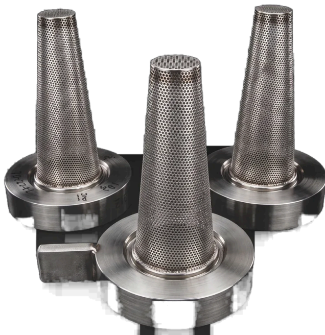
Conical and truncated-cone elements. Fitted between flanges on a spool piece and removed once the system has been cleaned.
